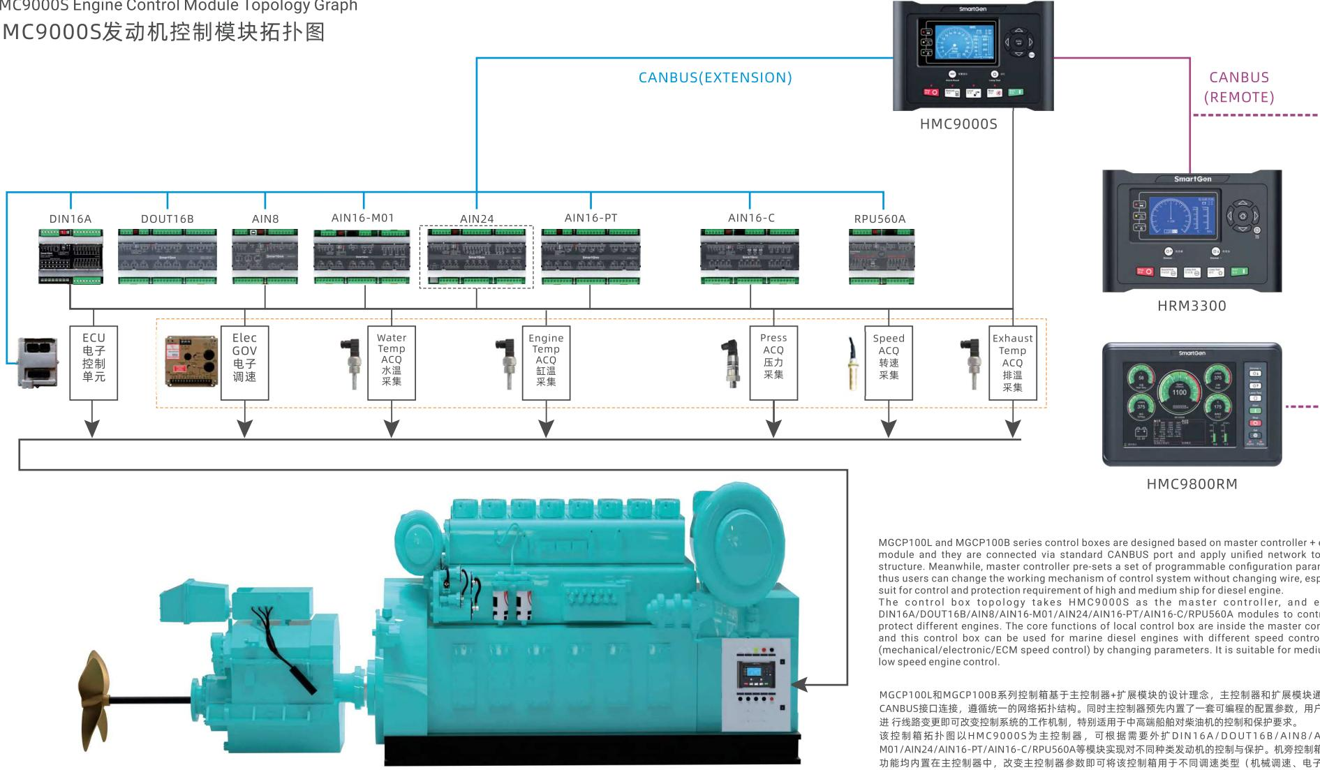
MGCP100L and MGCP100B series control boxes are designed based on master controller + expand module and they are connected via standard CANBUS port and apply unified network topology structure. Meanwhile, master controller pre-sets a set of programmable configuration parameters, thus users can change the working mechanism of control system without changing wire, especially suit for control and protection requirement of high and medium ship for diesel engine.
