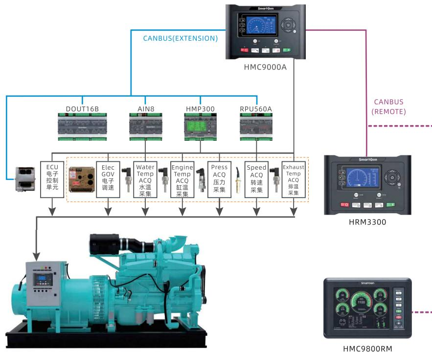
The control box topology takes HMC9000A as the master controller, and expand DOUT16B/AIN8/HMP300/RPU560A modules to control and protect different engines. The core functions of local control box are inside the master controller, and this control box can be used for marine diesel engines with different speed control types (mechanical/electronic/ECM speed control) by changing parameters. It is suitable for high and medium speed engine control. It is widely used for large and medium diesel engine.
